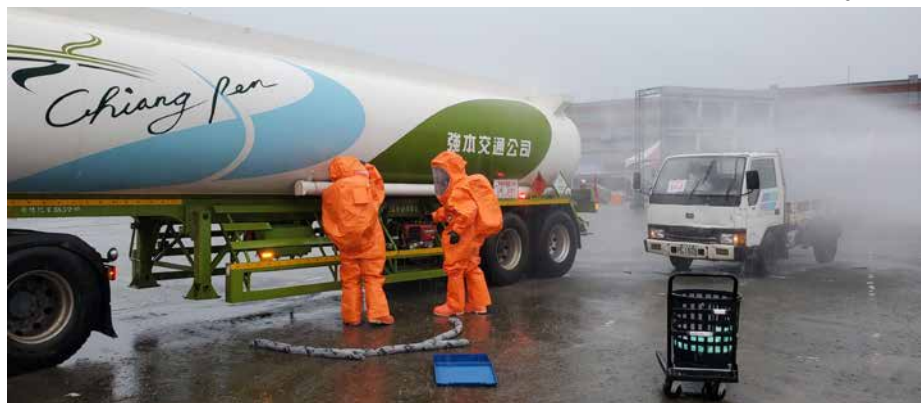
Using a leak sealing lance set to stop the leaks.
