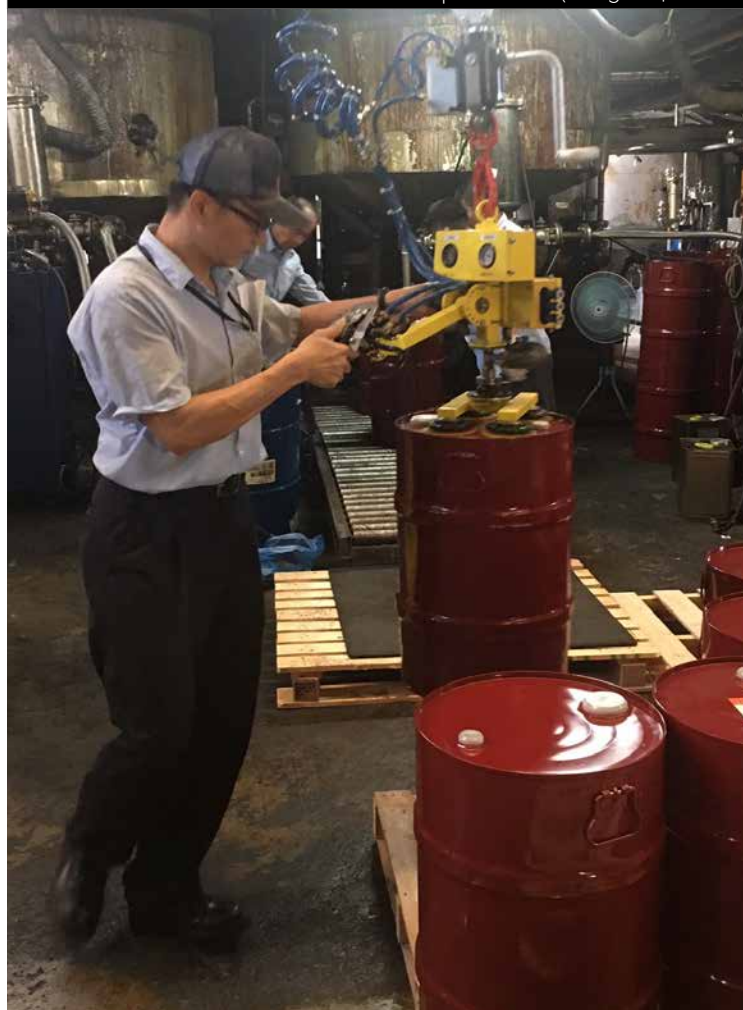
After Improvement (using suspended boom): September 7th, 2020
