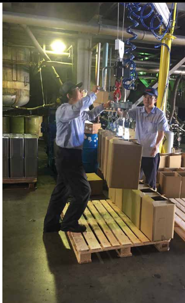
After Improvement (using suspended boom): September 7th, 2020
